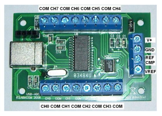
Connecting signals to the ADC make sure signals are within the "Absolute Maximum Ratings" of the LTC2309 to prevent damage.
