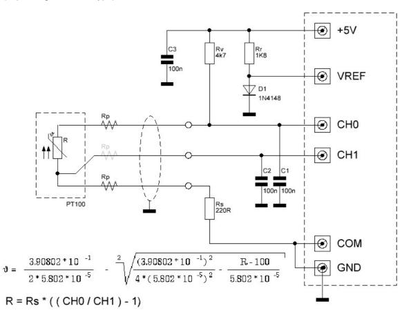
As each temperature channel needs two voltage channels, up to four PT100 can be connected to one module. The resistance R and the temperature must be calculated from the channel voltages by the software being used. Our software RealView and ProfiLab Expert is equipped with components that do the calculation, delivering temperature values directly.
