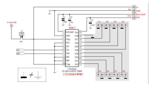
The analogue part consists of a high-quality ADC (Linear Technologies LTC2309) with internal voltage reference.
