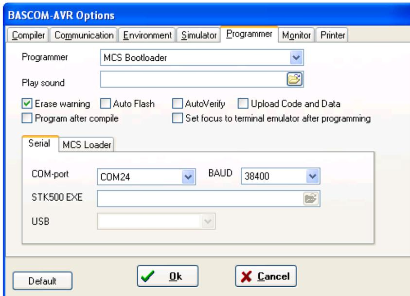
The virtual COM port (VCP) is installed by the device driver and can be found in the Windows Device Manager. It uses 38400 Baud transfer rate. All software options like 'Reset via DTR' can be used.
