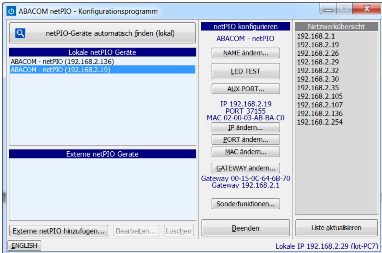
The network configuration tool (netPIO\_config.exe) is the same for any ABACOM netPIO product. It must be executed on a Windows-PC system which is connected to the same local network as the new netPIO device.
