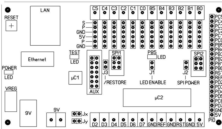
Dimensions 70mm x 120 mm (fits into WAGO DIN rail PCB carrier WAGO 288-600)
