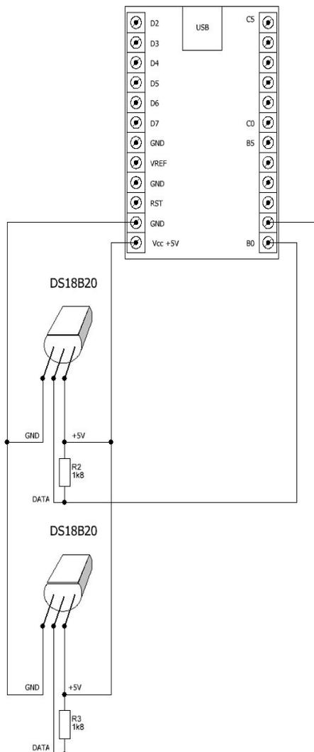
This chapter shows wiring diagrams using the USB-μPIO module. The can be found as well on the netPIO network module, with same functionality and arrangement.
