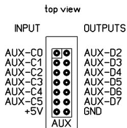
The AUX port pin-out from the component side,
