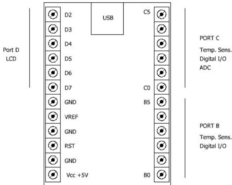
This chapter shows wiring diagrams using the USB- $\mu$ PIO module. The can be found as well on the netPIO network module, with same functionality and arrangement.
